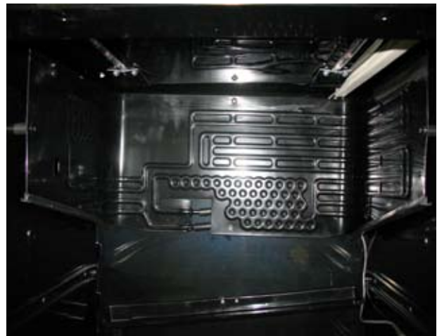
Figure 3.10: U-shaped evaporator plate used in the 6SBARE Typical low charge or system leak on this evaporator style will have a frost pattern that is only on the left hand side of the plate, not full across the plate.
