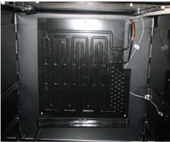
Figure 3.9: Multi-purpose evaporator plate used in the 8SWCE, 8SBARE, 6ORDE & 8ORDE
