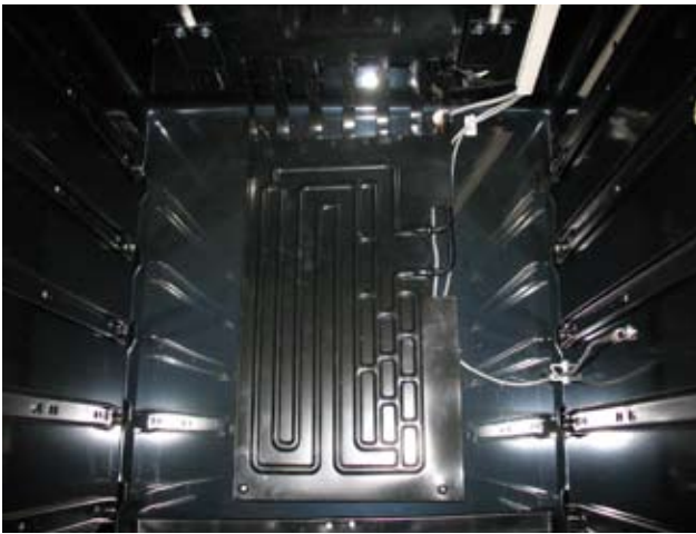
Figure 3.9: Vertical right angle evaporator plate used in the 30WCM & 3BARM
